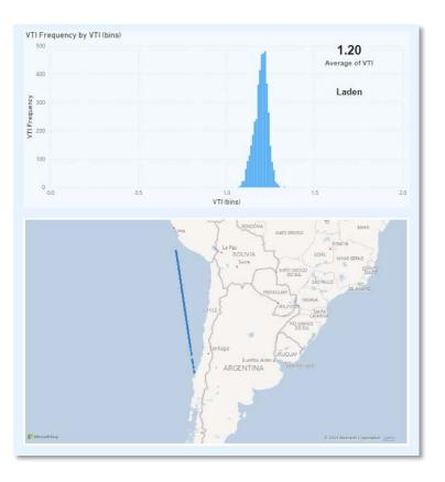
Average VTI of 1.20 indicate hull and/or propeller fouling
